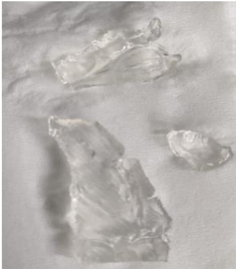
Figure 13. The photo on the PMAA-PIB8-20 sample swollen at pH 10 after its disintegration during the attempt for mechanical test
